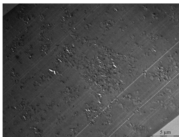
Figure 1 TEM micrograph of the cross section of a composite PI film containing 3 wt % of PANI.
